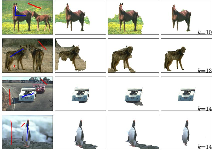
**Fig. 9.** The results of segmentation based on the geodesic distance, the  $k$ -max distance and the random walker technique. The input images with the seeds (first column), the results for the random walker (second column), the results for the geodesic distance (third column), the results for the  $k$ -max distance (fourth column).
