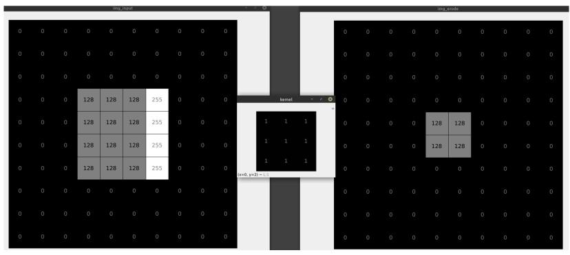
Idea of binary morphology can be extended to gray/color images with the use of max (Dilation) and min (Erosion) operation
