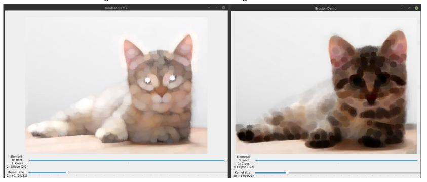
Analogous way: a morphological gradient is the difference between a dilation and an erosion
