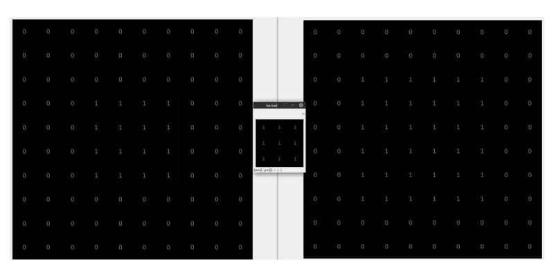
Opposite of erosion: a pixel element is '1' if at least one pixel under the kernel is '1'.
