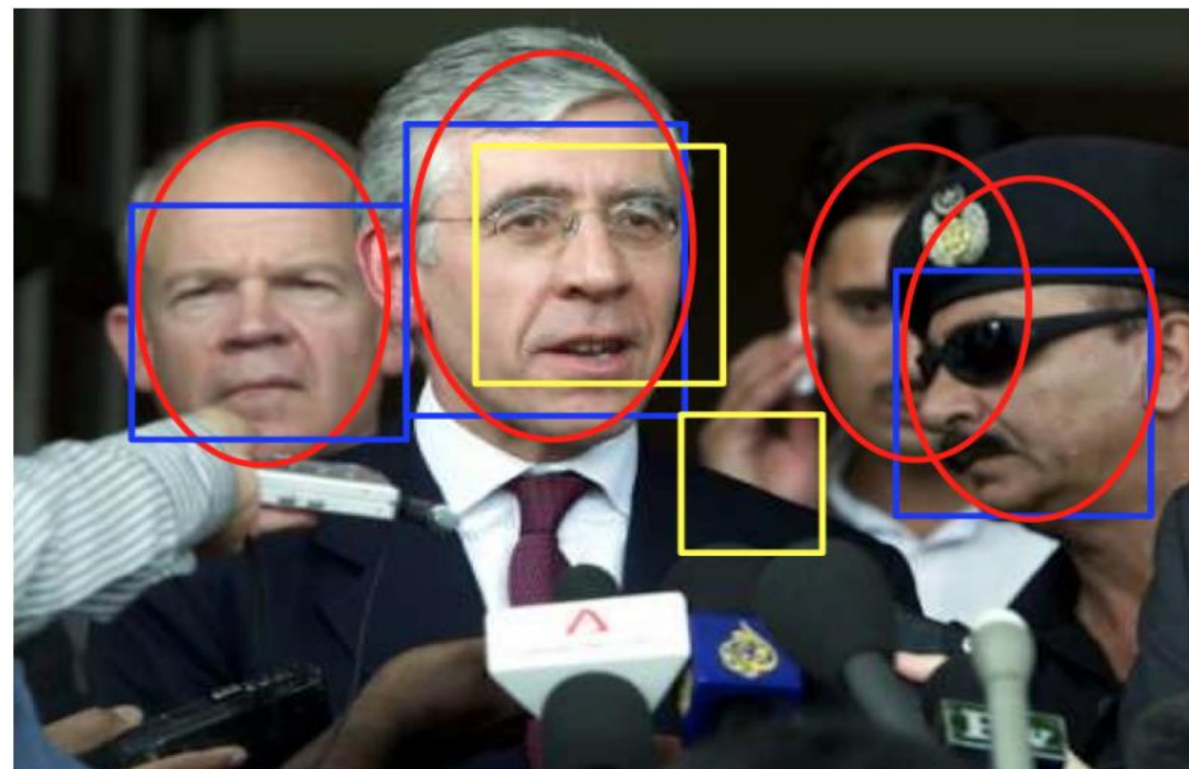
Figure 8. Matching detections and annotations. In this image, the ellipses specify the face annotations and the five rectangles denote a face detector's output. Note that the second face from left has two detections overlapping with it. We require a valid matching to accept only one of these detections as the true match, and to consider the other detection as a false positive. Also, note that the third face from the left has no detection overlapping with it, so no detection should be matched with this face. The blue rectangles denote the true positives and yellow rectangles denote the false positives in the desired matching.
