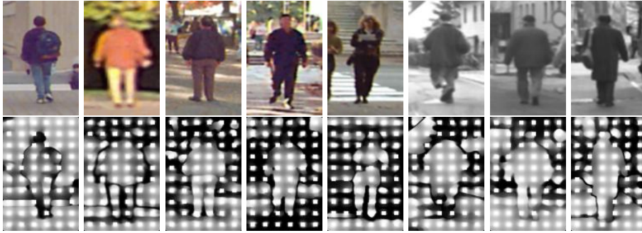
Fig. 5. The visualization of proposed descriptors of pedestrian images. The value of temperature is depicted by the level of brightness. The features are designed with the following parameters: the size of blocks 15 \times 15 ; the time t = 150 (the number of iterations for the transfer of temperature), the size of temperature sources = 5 \times 5 .
