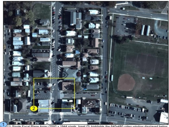
(1) Single Focal Plane Array (2552 x 1944 pixels). Inset (2) highlights the 640x480 video window displayed below.
