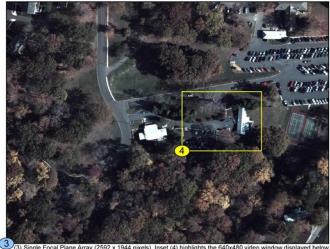
(3) Single Focal Plane Array (2552 x 1944 pixels). Inset (4) highlights the 640x480 video window displayed below.
