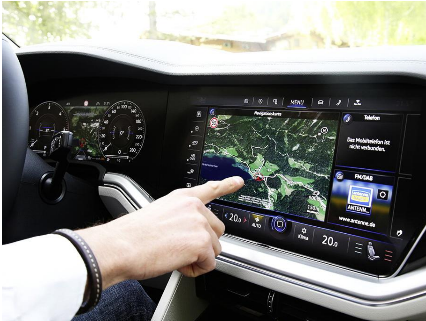
VW Touareg Innovision Cockpit with high-res displays placed in the head unit and the instrument cluster replacing the classic elements in front of the driver
