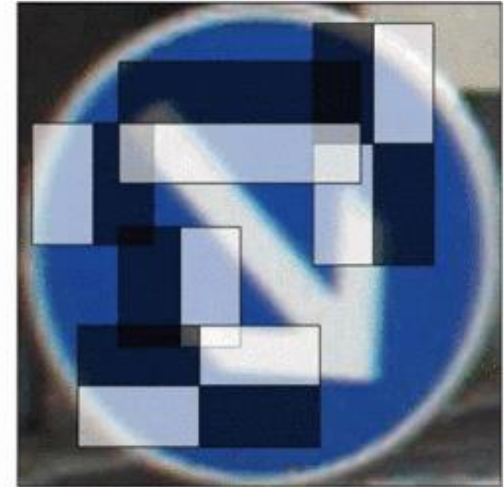
Five most significant Haar features selected for the first stage of each of the 3 trained detectors
